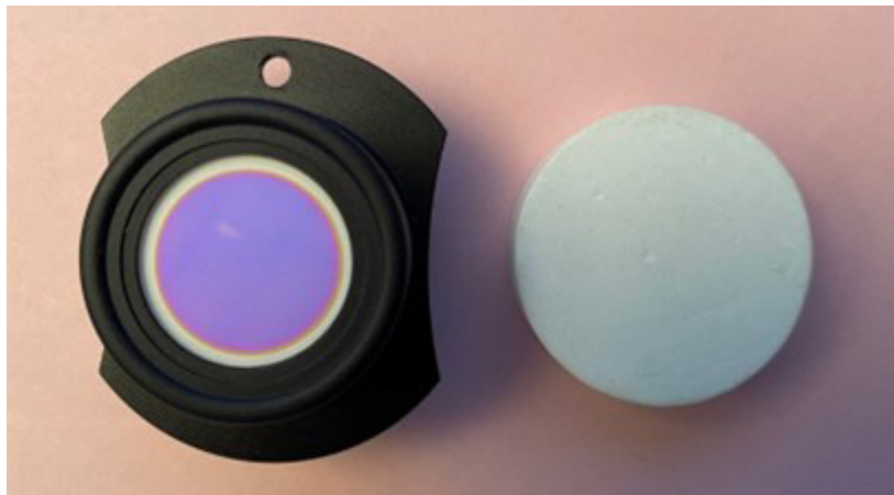
Figure 9. Protected (left) and unprotected (right) R99 reflectance standards
